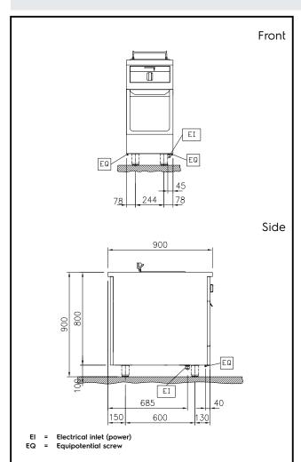
Electric Supply voltage: 400 V/3N ph/50/60 Hz Total Watts: 5.4 kW **Key Information:** Number of wells: Usable well dimensions (width): 240 mm Usable well dimensions 135 mm (height): Usable well dimensions 380 mm (depth): Well capacity: 6 lt MIN; 7 lt MAX Thermostat Range: 100 °C MIN; 180 °C MAX External dimensions, Width: 400 mm External dimensions, Depth: 900 mm External dimensions, Height: 800 mm Net weight: 70 kg On Base;One-Side Configuration: Operated
